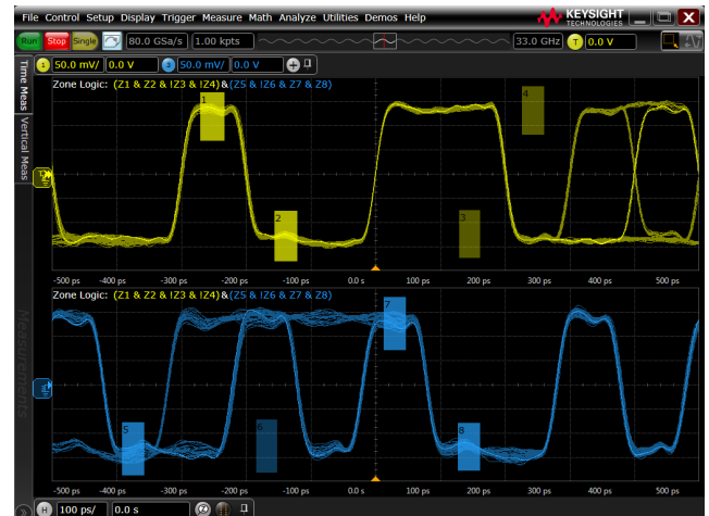
Draw up to eight "must intersect" or "must not intersect" zones to trigger on a specific event and condition.
